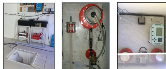
Figure 7: From top to bottom, google earth map showing the location of the laboratory at the TVA (rectangle in the inset), in Lanzarote. Several pictures taken inside the TIM-LGL showing the observational facilities and some scientific instruments installed: (left) water tube tiltmeter; (center) water-tube tiltmeter, extensometer; (right) gravimeter, vertical pendulums, seismometer.
